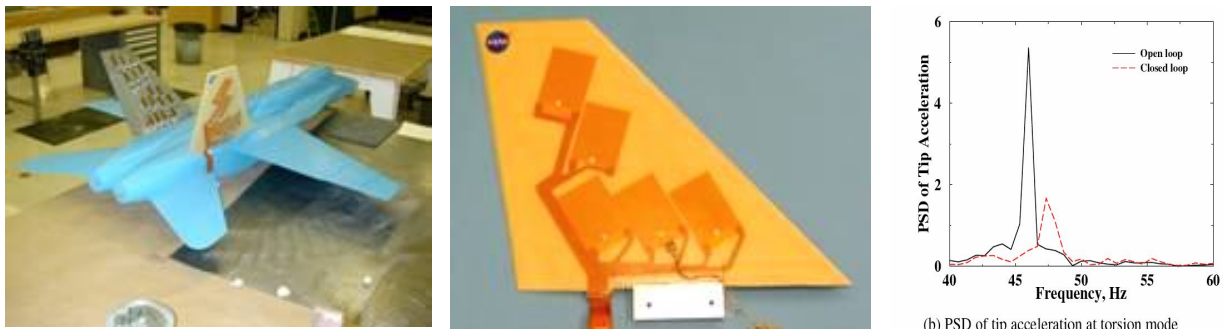
Figure 3: actuated tail-buffet using MFC actuators
